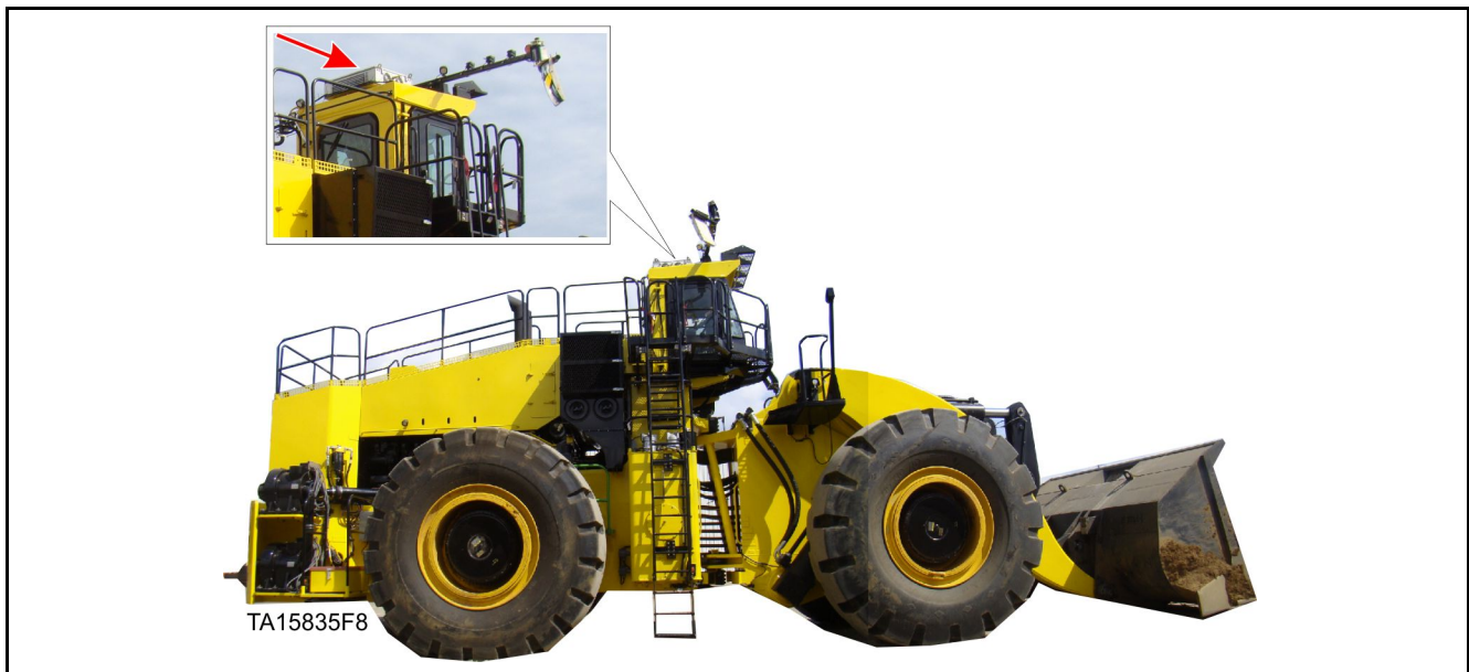
Figure 2. Air conditioner unit location (typical)
